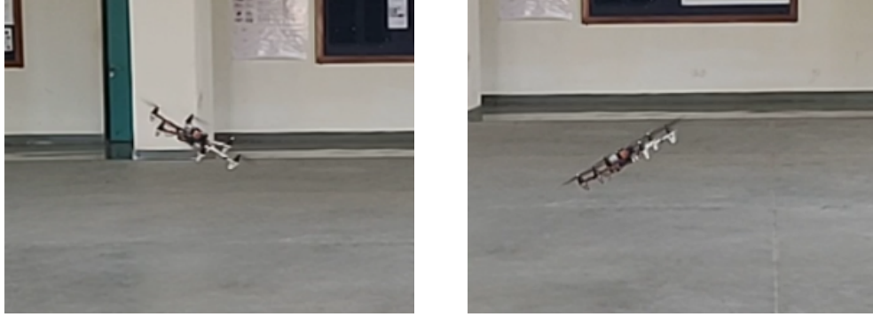
(A) Hexarotor with a positive pitch angle. (B) Hexarotor with a negative pitch angle.
