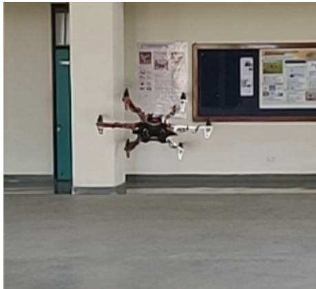
(A) Hexarotor with positive roll angle.
