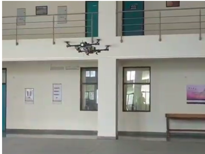
FIGURE 4.27: Variable-pitch quadrotor in hover state.
