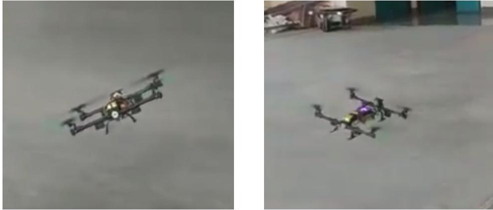
(A) Quadrotor with negative roll angle. (B) Quadrotor with positive roll angle.
