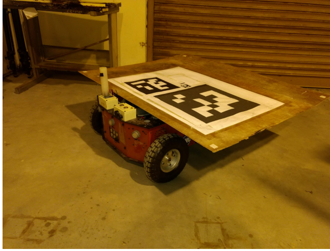
Figure 18: Ground robot with the landing platform and the compound marker.
