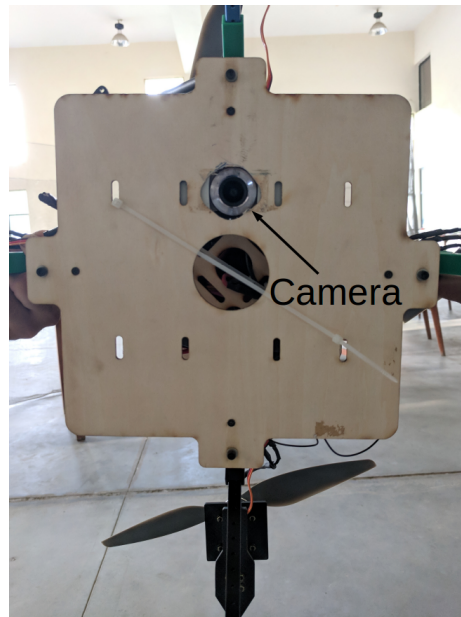
Figure 17: The camera fixed on the tilt-augmented quadrotor.
